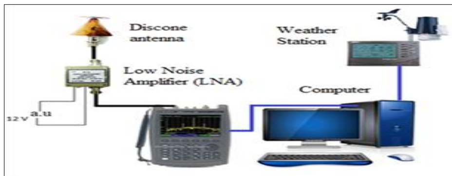
Figure 3. The instruments set up for observation work
